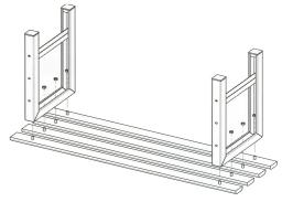
Turn over the bench and secure the 2 cross bars in the outer holes of the legs with 4 flanged screws TE 8x16 with nut.
